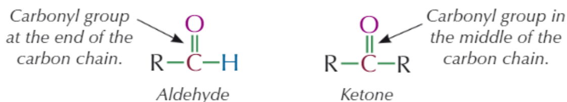
Figure 1: The difference between an aldehyde and a ketone. 'R' represents a carbon chain of any length.
